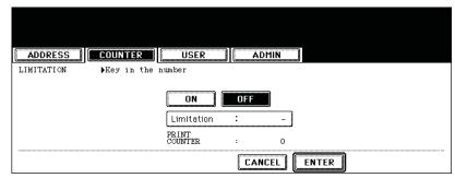
Press the [ON] button to enable the output limitation for this department code. When you select the [ON] button, press the "Limitation" field and enter the maximum number of the outputs for this department code using the digital keys. You can enter up to "99999999". If you do not set the output limitation for outputs, press the [OFF] button.
